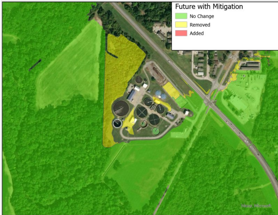
Figure 14: Current versus with mitigation floodplain plots
