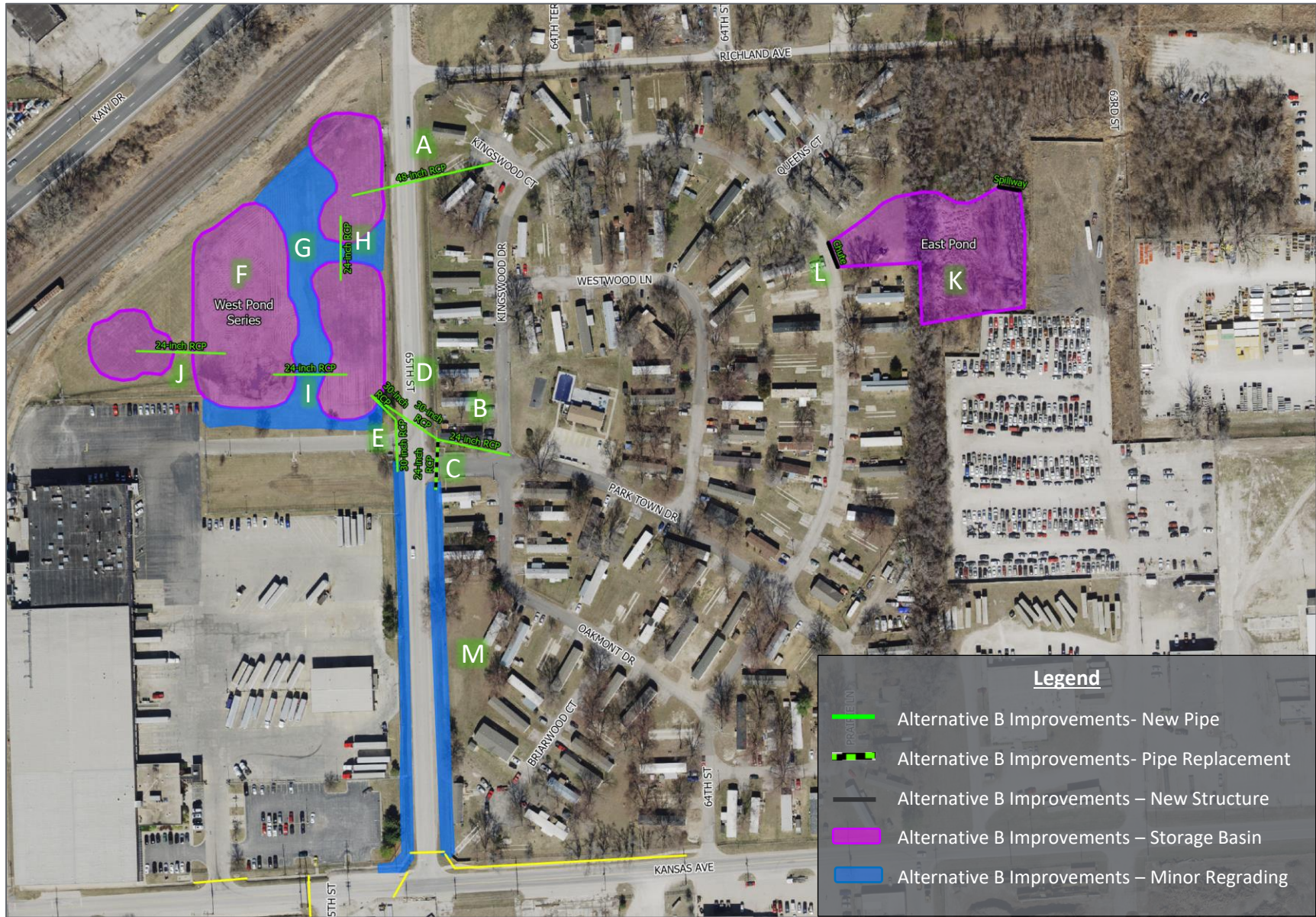
FIGURE 16 - IMAGE OF ALTERNATIVE B IMPROVEMENTS
