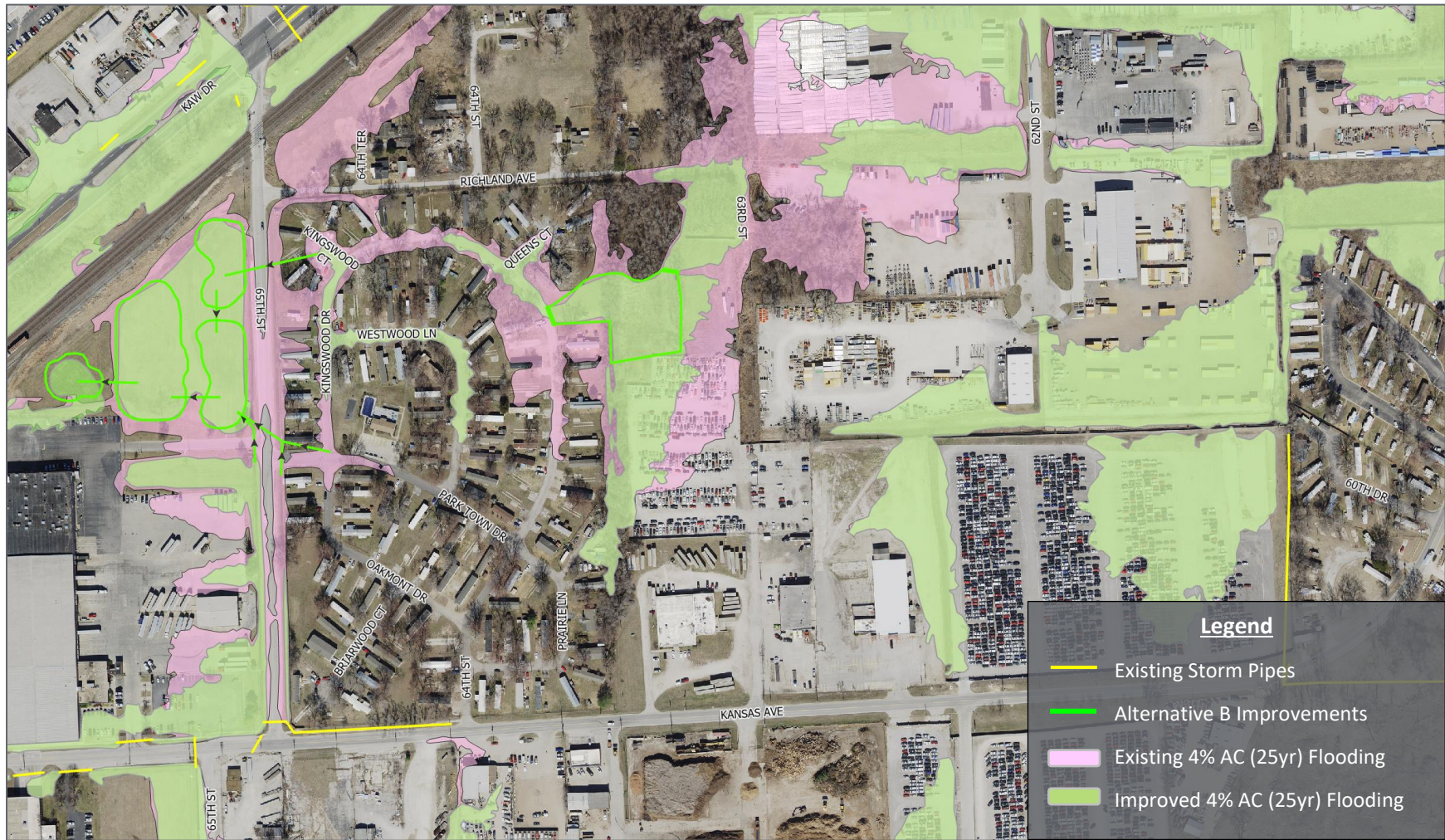
FIGURE 18- ALTERNATIVE B FLOOD COMPARISONS FOR EXISTING LAND USE AND 25-YR STORM EVENT
