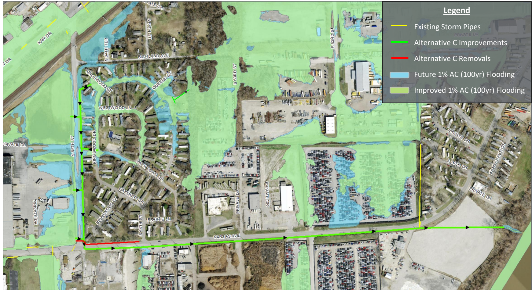
FIGURE 27 - ALTERNATIVE C FLOOD COMPARISONS FOR FUTURE LAND USE AND 100-YR STORM EVENT
