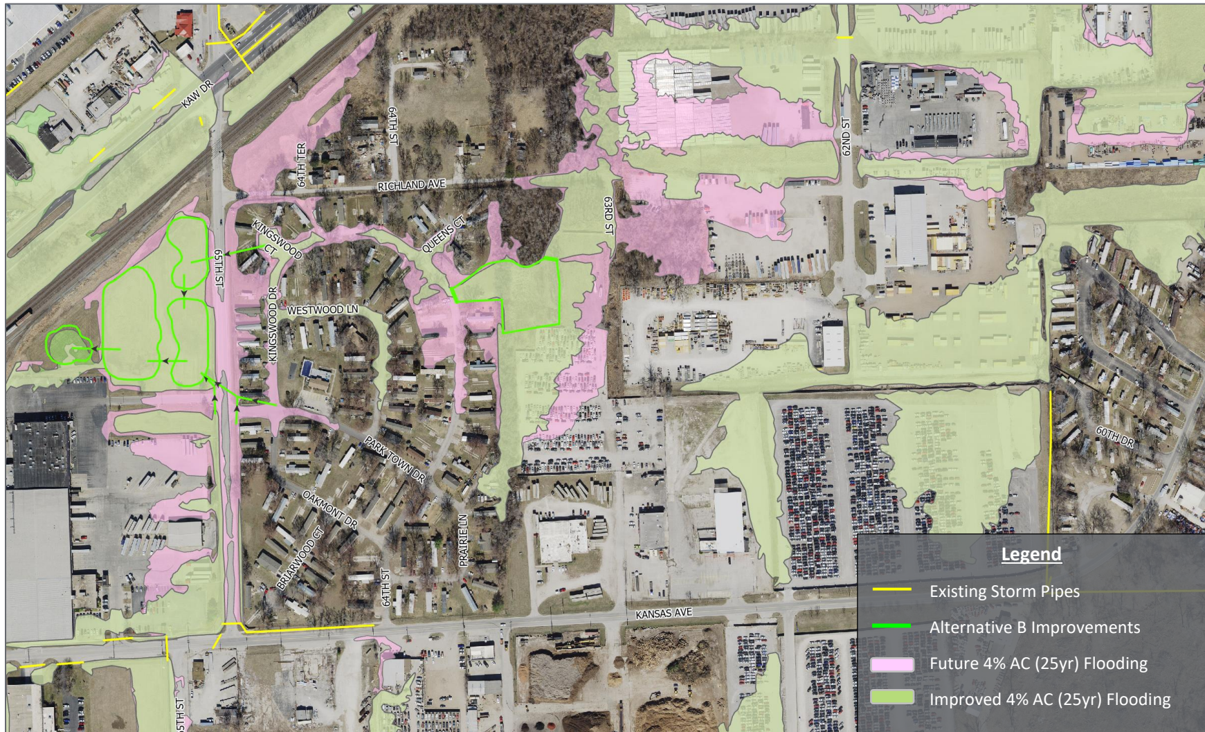
FIGURE 20 - ALTERNATIVE B FLOOD COMPARISONS FOR FUTURE LAND USE AND 25-YR STORM EVENT
