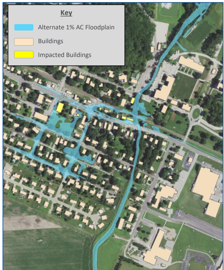
FIGURE 9 - DOWNSTREAM FLOODING ASSOCIATED WITH 50YR FLOOD DETENTION DAM
