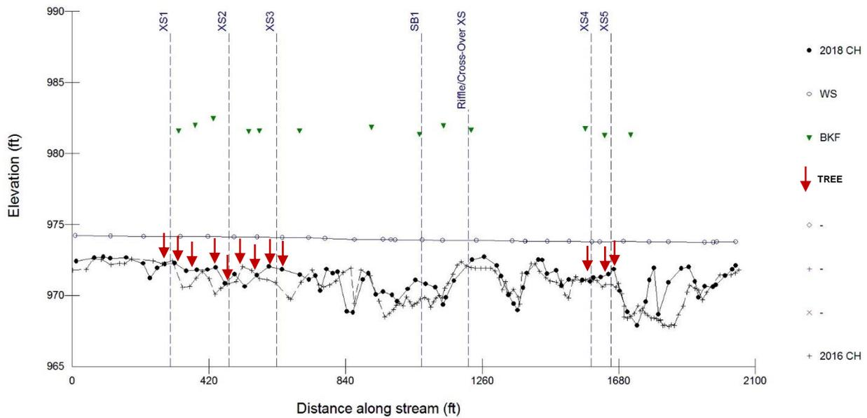
Figure 5. Example Longitudinal Profile from Reach 6, March 2016 and March 2018. Note: CH: thalweg; WS: water surface; BKF: bankfull; XS: cross section; SB: study bank; TREE: installed woody revetment
