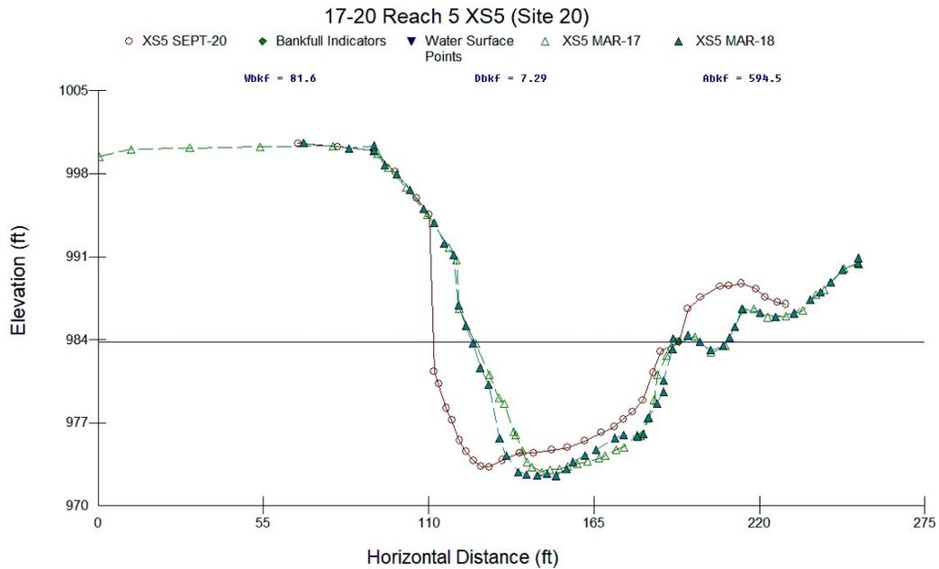
Figure C.5. Reach 5 XS5 at Site 20 Survey, March 2017, March 2018, and September 2020. This cross section is between revetments 5 and 6 (of 7) that was washed out by 2020.
