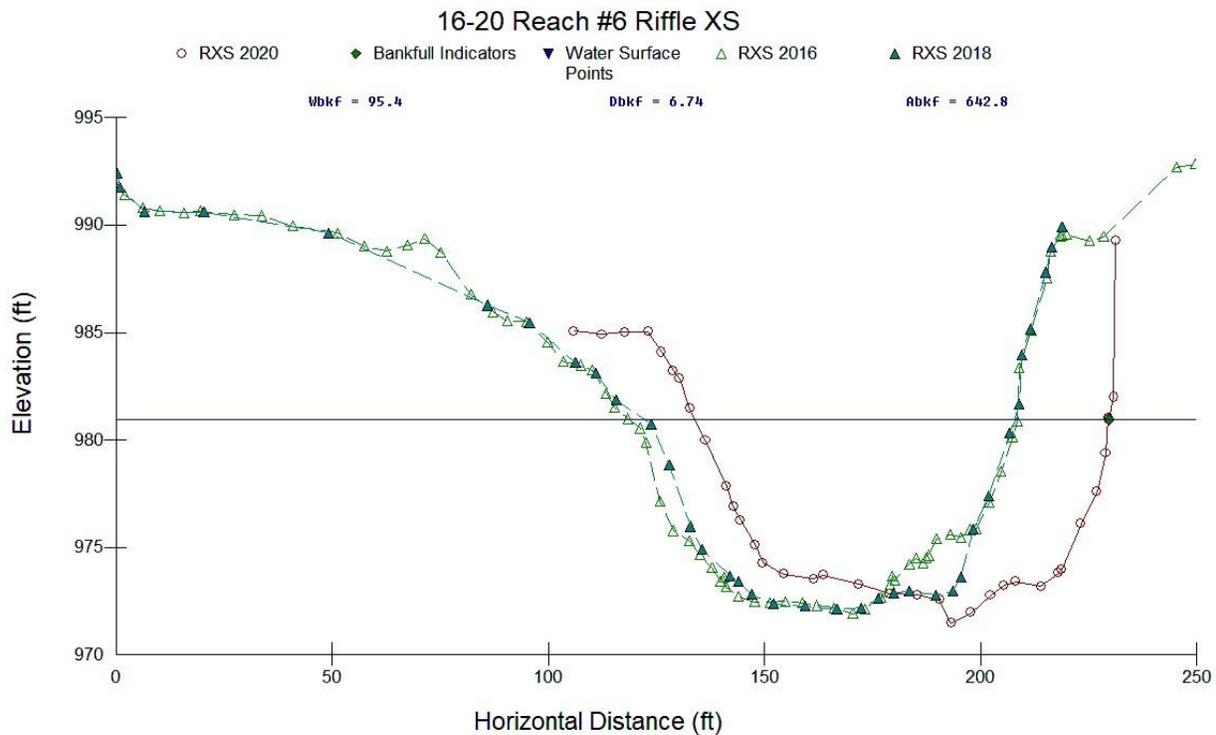
Figure 6. Example Cross-Over Cross Section (XS) Survey from Reach 6, March 2016, March 2018, and May 2020. The solid blue line indicates the suspected bankfull elevation.
