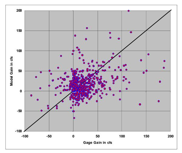
Figure 3 – Scatter diagram of computed and measured (gaged) gains between Dodge City and Kinsley using 1-layer representation of BBGMD5 model.
