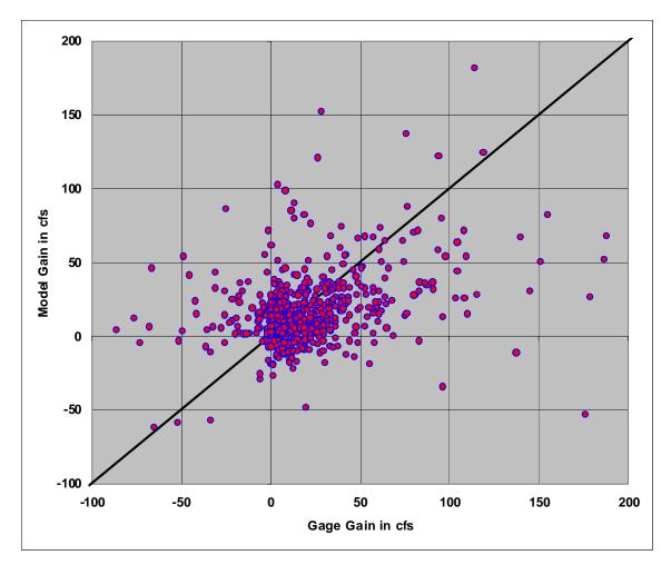
Figure 4 – Scatter diagram of computed and measured (gaged) gains between Dodge City and Kinsley using alternative 1-layer representation of BBGMD5 model.
