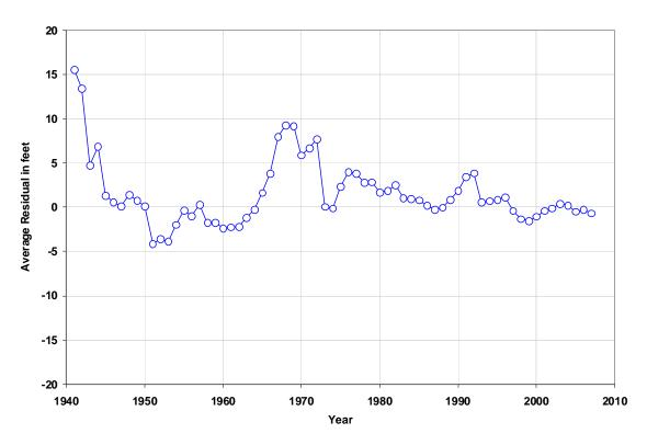
Figure 2 – Average residual for groundwater levels in GMD 5 area using alternative 1-layer representation of BBGMD5 model.
