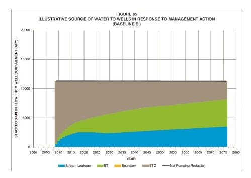
Figure 5 – Illustration of pumping impacts on stream flow/leakage and ET using the BBGMD5 model.
