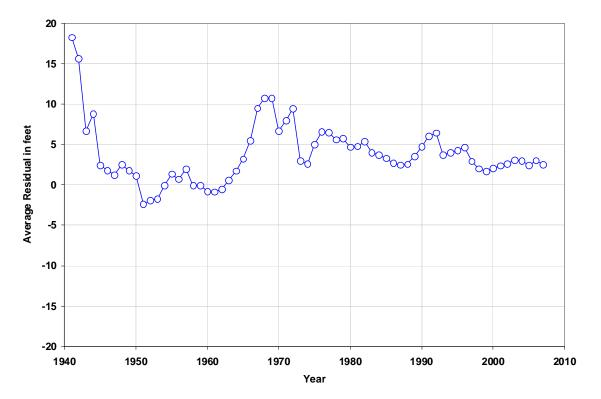
Figure 1 – Average residual for groundwater levels in GMD 5 area using 1-layer representation of BBGMD5 model.
