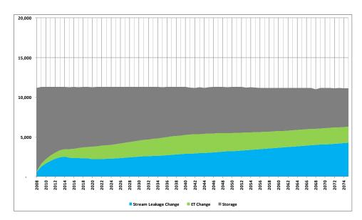
Figure 6 – Illustration of pumping impacts on stream flow/leakage and ET using the alternative 1-layer representation of the BBGMD5 model.
